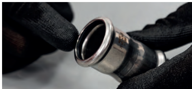
Figure 35 – Checking the sealing ring
