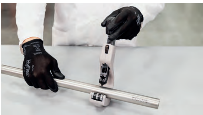
Figure 26 - Cutting the pipe to length
