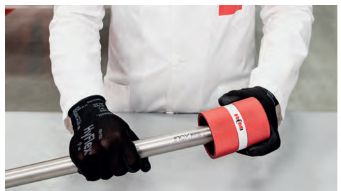
Figure 27 - Deburring the pipe
