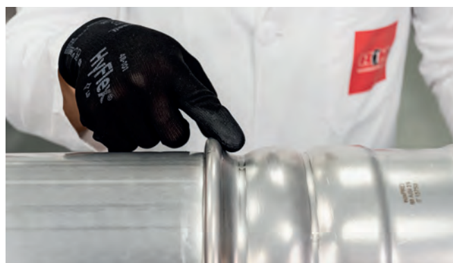
Figure 41 – Visual inspection of oversized pressing
